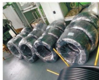
Flexible pipes for tractor “Belarus” air brake systems made of polyamide composite “Etamid EA-2EU (T)” (TU VU40084698.267-2014). More than 100 km of pipes were produced
