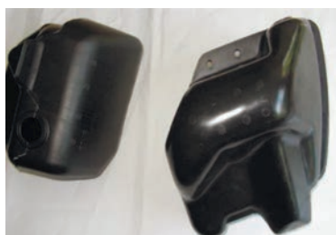
Gasoline vapor separator made of polyamide composite “Etamide EA-EU (V)” (TCBY40084698.267-2014). JSC Avtovaz (Tolyatti, Russian Federation) produced more than 50,000 separators
